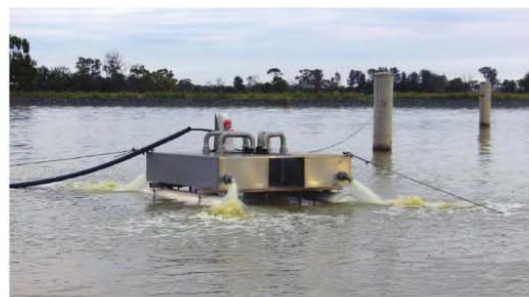
The Andzac Aerator in operation at Kyabram.
